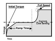
Figure APP 1.2: Voltage Ramp with Current Limit
