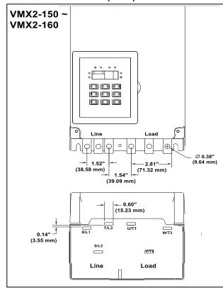
Figure 2.6.3 Critical clearances for bus tab connections
