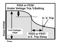
Figure 5.6.6.b: Under Voltage Trip
