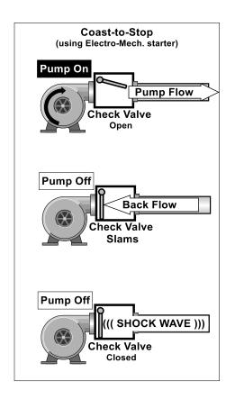
Pump-Flex® Deceleration (Soft Stop) is a unique feature of Motortronics Solid State Soft Starters. It provides a slow decrease in the output voltage, accomplishing a gentle decrease in motor torque during the stopping mode. This is the **OPPOSITE OF BRAKING**, in that it will take **longer** to come to a stop than if the starter were just tuned off.
