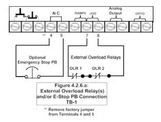
4.2.6.a External Overload Relay Connection
