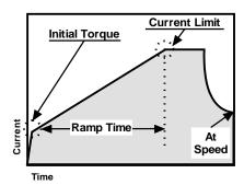
Figure APP 1.3: Current / Torque Ramp
