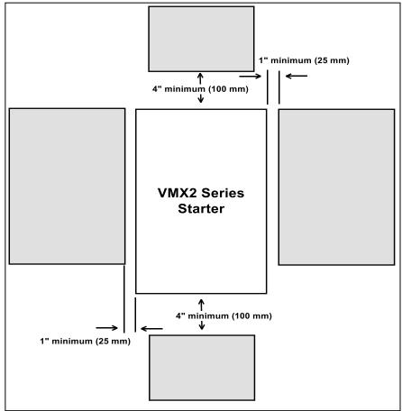
Figure 2.5: VMX2 minimum mounting clearances
