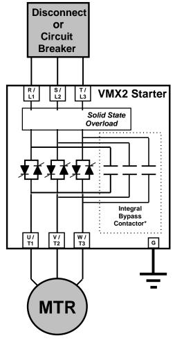
Figure 4.1: VMX2 Power Connections
